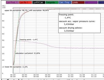
LyoControl: freezing point determination with LyoLogplus
