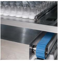
The shelves move up. The LyoShuttle robot drives behind the shelf package. The shelf to be unloaded moves on constant loading level.
