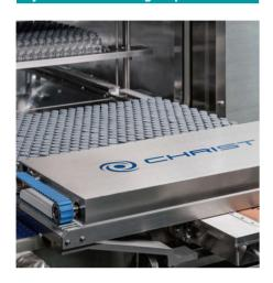
The LyoShuttle robot pushes the vial package on the shelf.
