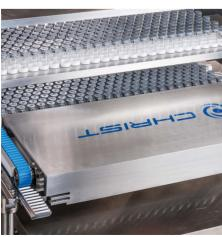
The LyoShuttle robot pushes the vial package out of the freeze dryer.
