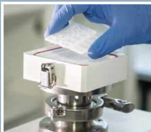
CCIT of Blow, Fill, Seal containers, vacuum decay test method
