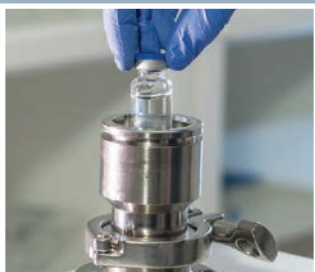
CCIT of vial, vacuum or pressure decay testing methods
