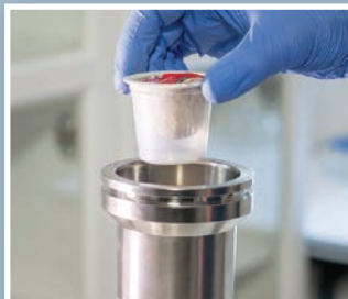
CCIT of capsule, vacuum decay test combined with lid deflection method
