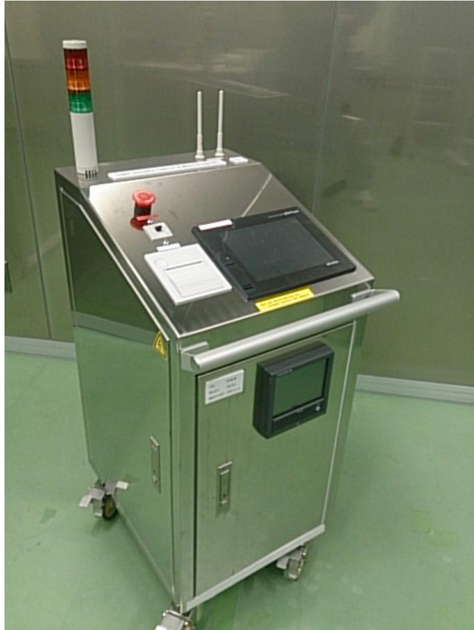
Start room decontamination from the unclassified area. No cables are needed. Communication is wireless with the HPG generator & distribution unit and sensor unit
